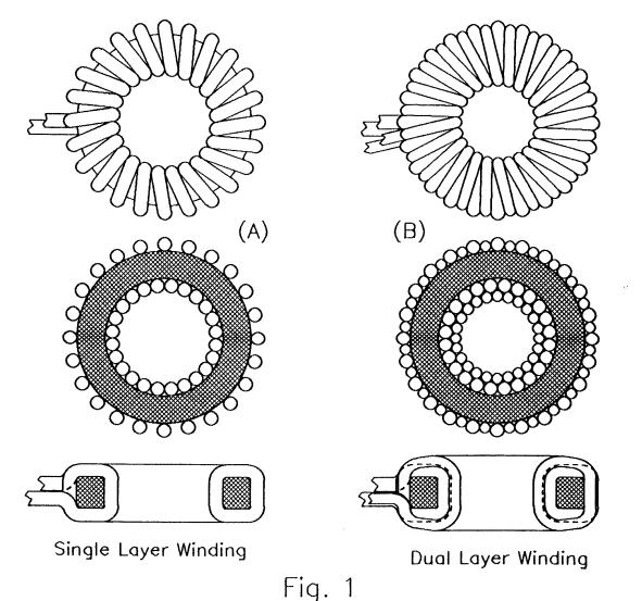
"Precision" Toroidal Windings
